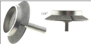
Beveled grinding wheel with a 120 degree bevel and a 10mm shank it is about 2-inches in diameter. Like all diamond grinders these and all others must be used in water.
