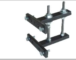
The slab grabber allows you to get the last slab out of any butt cut or small rock that you have or if you want to cut a thick slab in half by just centering it up and claming it in the fixture. It will adjust to hold a rock that is up to 5 inches tall. It will pay for it self in just a few cuts of your favorite rock.
